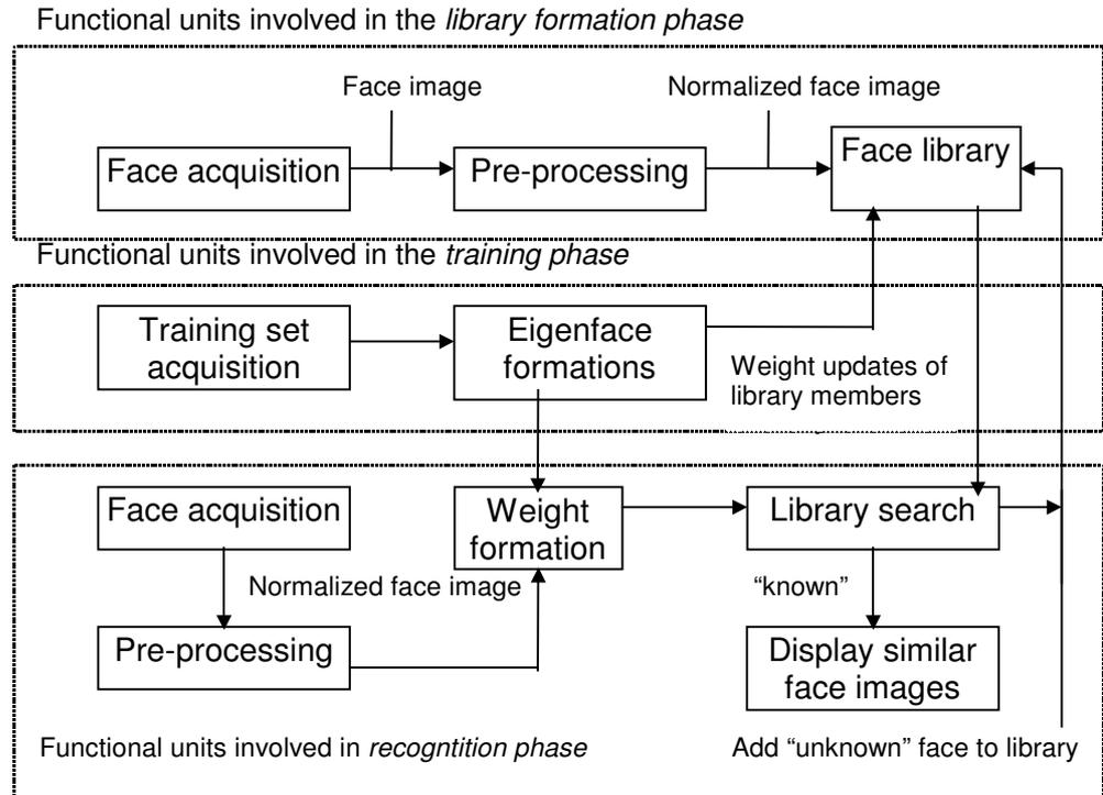
**Figure 3.3.** Functional block diagram of the proposed face recognition system.
