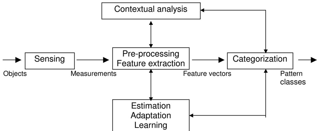
**Figure 2.2.** Functional block diagram of an adaptive pattern recognition system.
